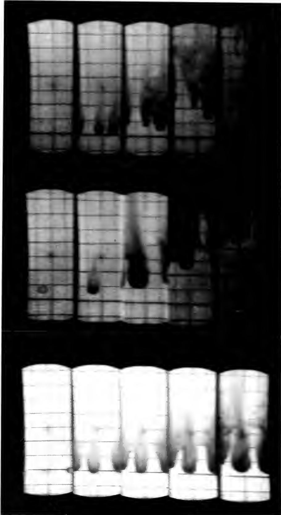
a. b. c. FIGURE 5. TYPICAL SHADOW PHOTOGRAPH SEQUENCES: a. D=2.06 mm, M_S=1.84 ; b. D=2.74 mm, M_S=2.01 ; c. D=.985 mm, M_S=1.90
